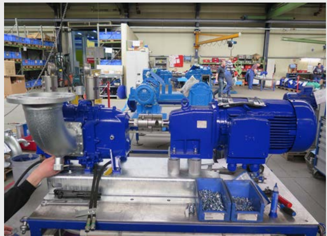
ROTEX® S-H with SPLIT hubs built into a rotary lobe pump
